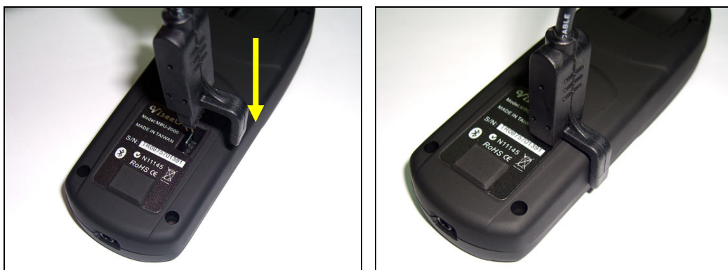
Gently plug the 10-pin connector into the CPU upgrade ports in the direction as shown
